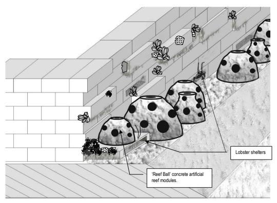
Presentation of wall above the waterline does not have to change yet biological attractiveness of wall below the waterline is significantly enhanced. Extended bricks should be random and do not have to be used throughout the whole wall.
